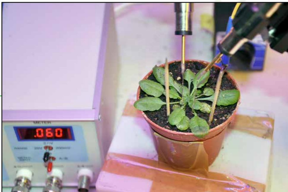
Figure 44: Measuring wound-induced electrical signals in a 5 week-old Arabidopsis rosette. (By courtesy of Prof. Edward Elliston Farmer, University of Lausanne.)
